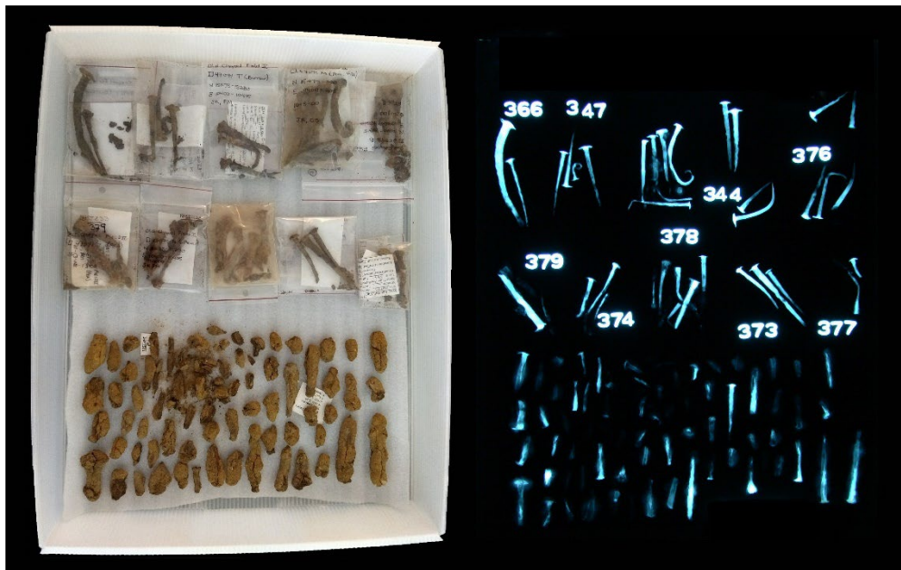
Figure 4-1. Example of proper layout of materials for x-ray. Small proveniences may be left in their respective bags (Morehouse, Rivers Cofield, and Doub, 2022).
